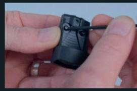
2 . Apply pressure with the hex wrench until you hear a click, indicating the pin has disengaged.
