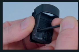
4. Once both pins have disengaged, you should be able to easily remove the battery cover.
