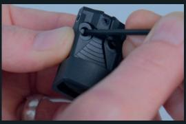
3. To repeat on the second pin, turn the sight around and repeat the process for the second pin, applying pressure at a 45-degree angle until you hear a click.
